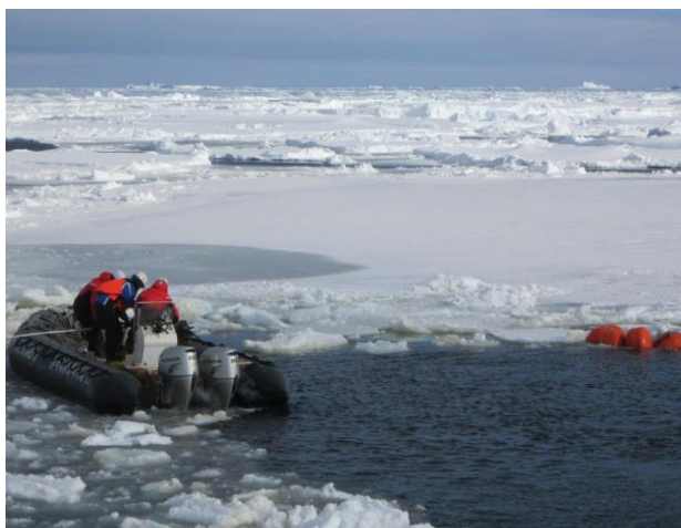
In the midst of sea ice, Araon crew aboard a Zodiac boat is retrieving the surfaced mooring device that was deployed a year ago and now loaded with important scientific data.
